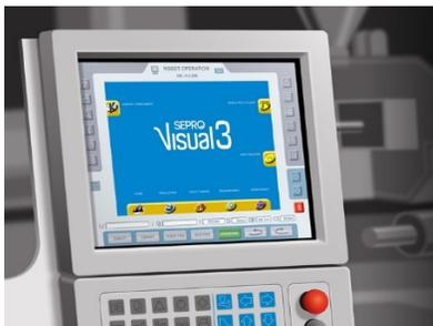
*Open Integration from Sepro allows the robot control interface to be presented on the molding machine HMI. Download a high-resolution file at:
